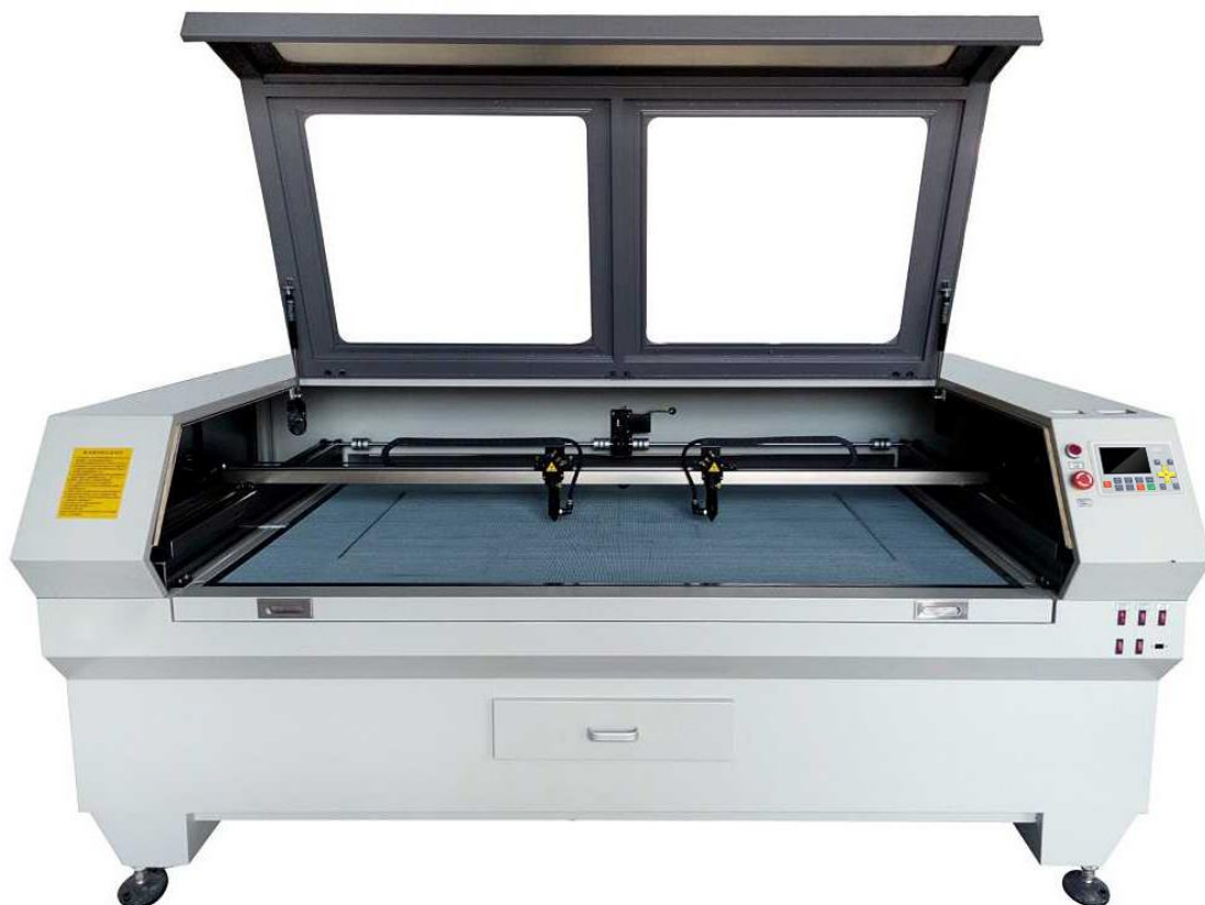
Figure7-6-3 Mutual Movable Double Laser Head Cutting
